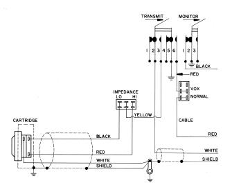
MODEL 444D-RK199S SWITCH WIRING FIGURE 2
